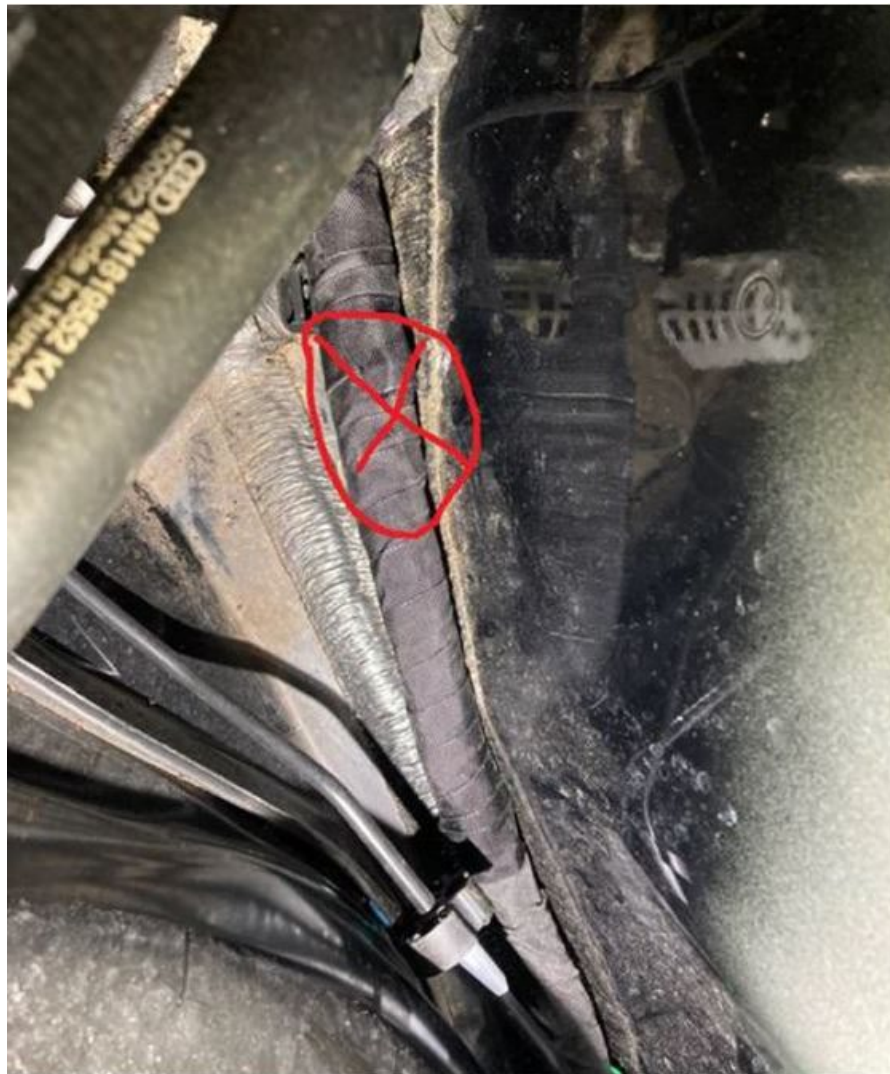
Figure 1. No external damage to the wiring harness can be seen.
