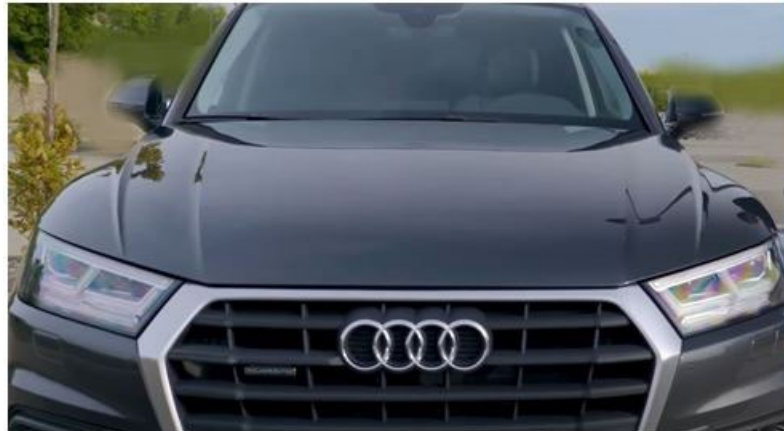
Figure 1: Rainbow-colored shimmer on the inside of lens.
