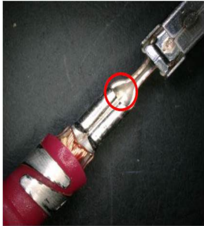
Figure 2. Improperly crimped wire.
