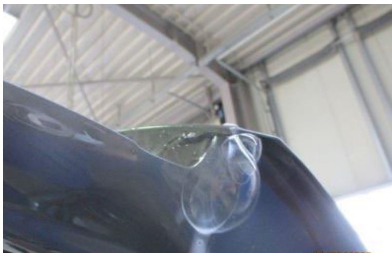
Figure 1. Bubble formation with compressed air applied internally.
