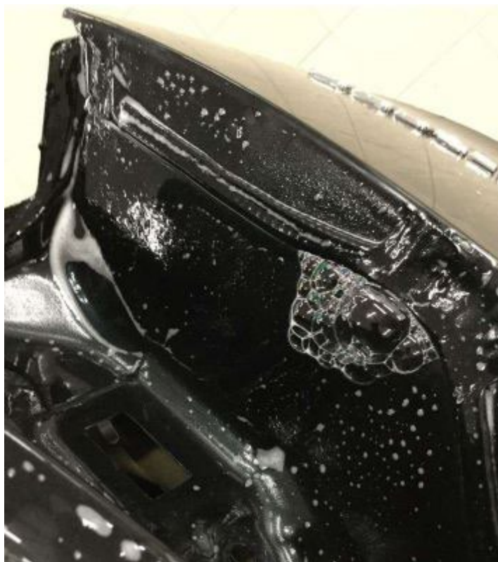
Figure 3. Bubble formation with compressed air applied internally.
