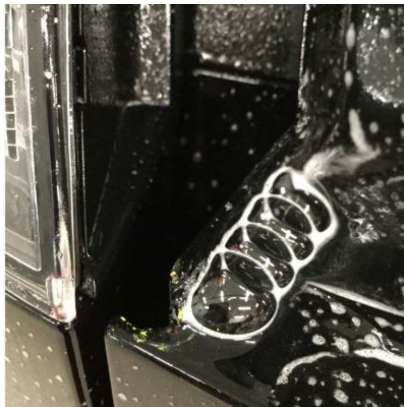
Figure 2. Bubble formation with compressed air applied internally.
