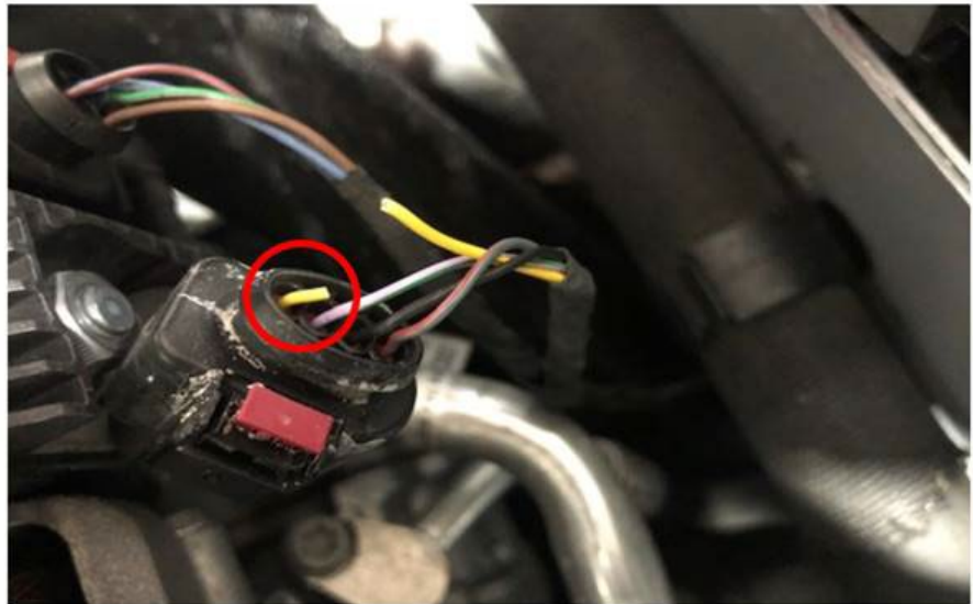
Figure 1. Wire is broken at G31 sensor.
