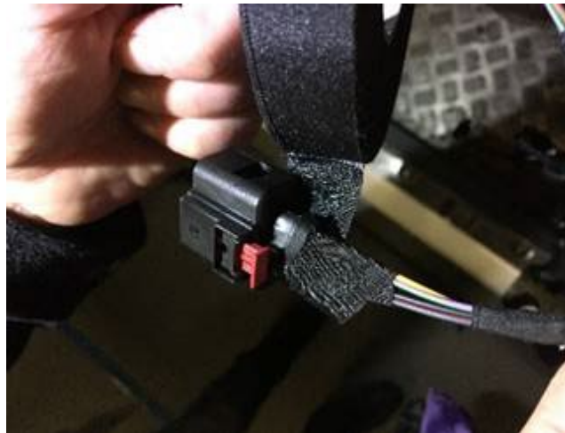
Figure 3. Wrapping the connector base.
