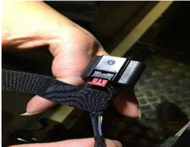
Figure 4. Wrapping the connector base part 2.
