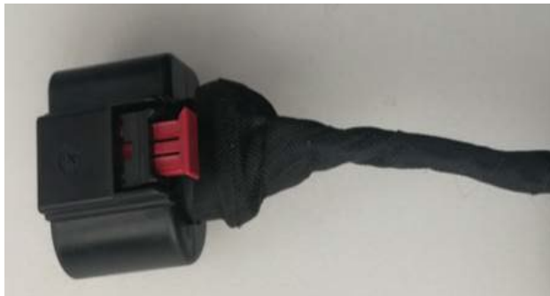
Figure 5. Completed harness wrapping.
