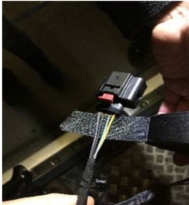
Figure 2. Harness is wrapped using textile tape 105 920 02.
