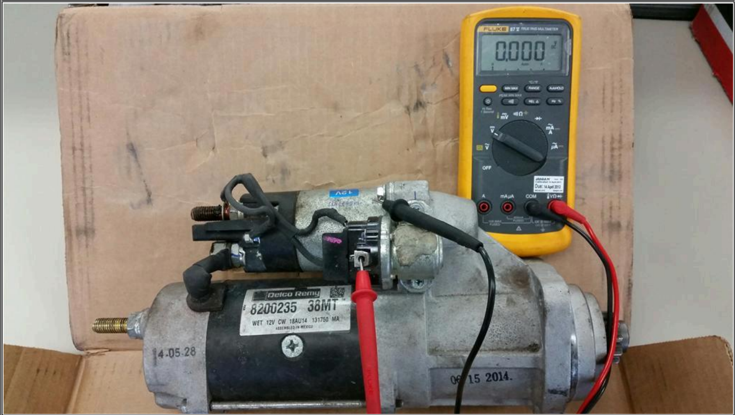
Figure 4: Starter IMS S terminal DVOM Hookup Location
