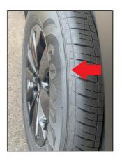
Sidewall waviness/indentations/undulations are common on radial tires and are more noticeable on tires with taller sidewalls. The higher the tire pressure, the more noticeable the effect will be. Be sure to set the tire pressures at the recommended tire pressure on the vehicle tire label.
