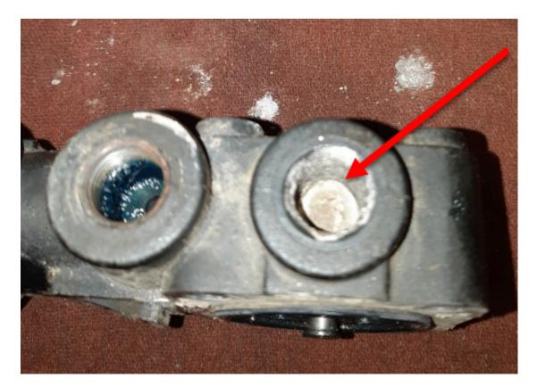
**1.** Verify the unit is equipped with a Barksdale leveling valve and that it is clogged.
