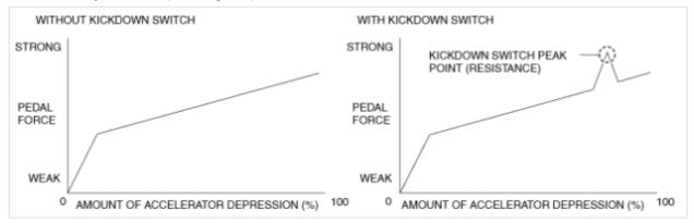
• Because the driver can determine the accelerator pedal depression amount from the change in the pedal depression (change in depression force), kick-down control is achieved.
