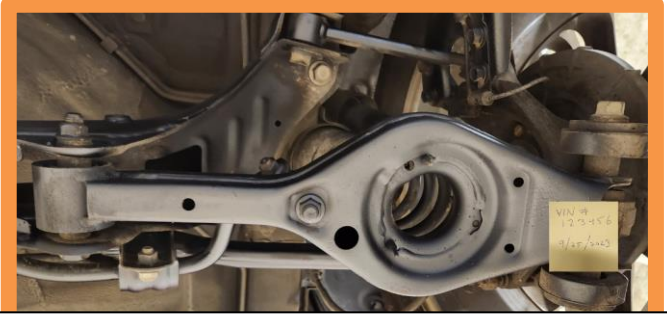
7. Left rear suspension components: lower control arm, upper control arm, assist arm.
