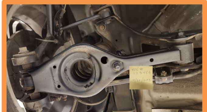
8. Right rear suspension components: lower control arm, upper control arm, assist arm.
