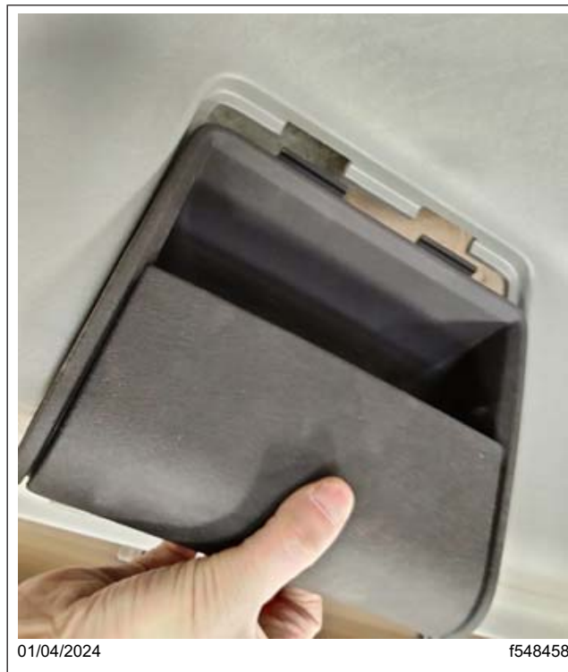
Fig. 13, Sunglasses Pocket Removal from the Overhead Console
