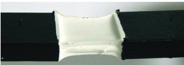
Sikaflex®-715 is a "cured" product and demonstrates good flexibility and retains its shape.
