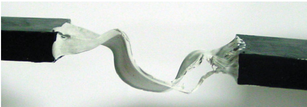
Traditional sealant has stringy, putty like substance and easily pulls apart and breaks.
