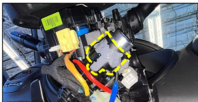
The ignition housing (D) shown above was removed for illustration purpose ONLY . Refer to the image below.
