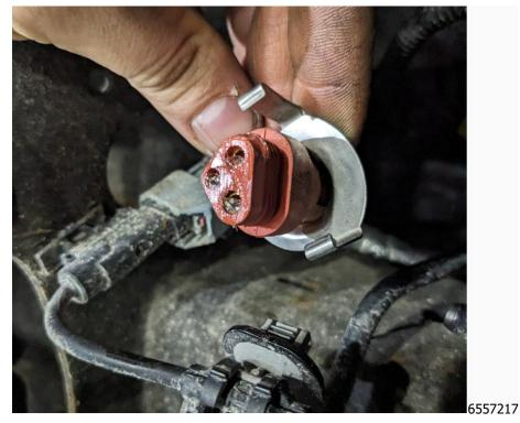
6. Apply dielectric grease as shown (a light coat applied by hand or brush to the end of the cord).
