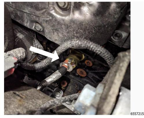
3. Locate the engine block heater through the opening in the wheel well liner.
