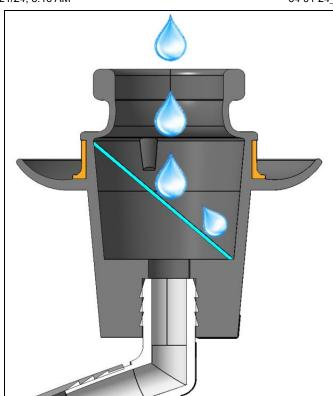
A ramp insert has been placed into the condensation drain plug, so the water drops falling into the condensate drain pipe are broken up- eliminating the drumming noise.
