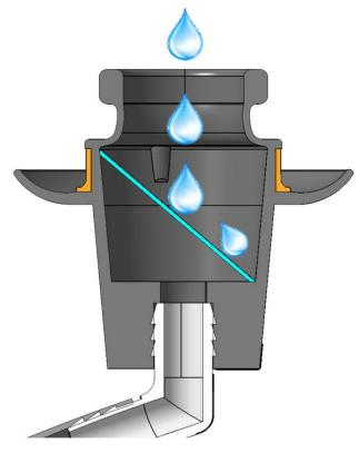
The condensation drain has been optimized and can be identified by a **WHITE DOT** or revision **INDEX 02** or higher.
