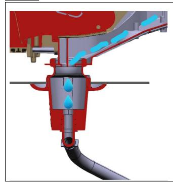
Warm temperatures combined with high air humidity may lead to the formation of condensate in the blower housing.
