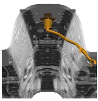
Replace the condensation water drain.
