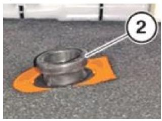
Prior to installing new drain into body from below apply lubricant to the top of the seal (2) where it contacts the heater box.
