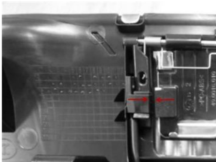
Figure 6. Excessive hall sensor to induction plate air gap.
