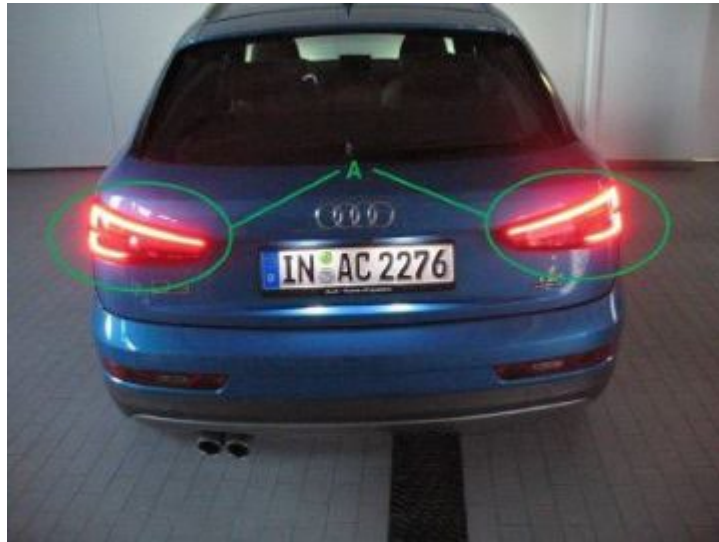
Figure 1. Rear lamp operation with rear lid closed.
