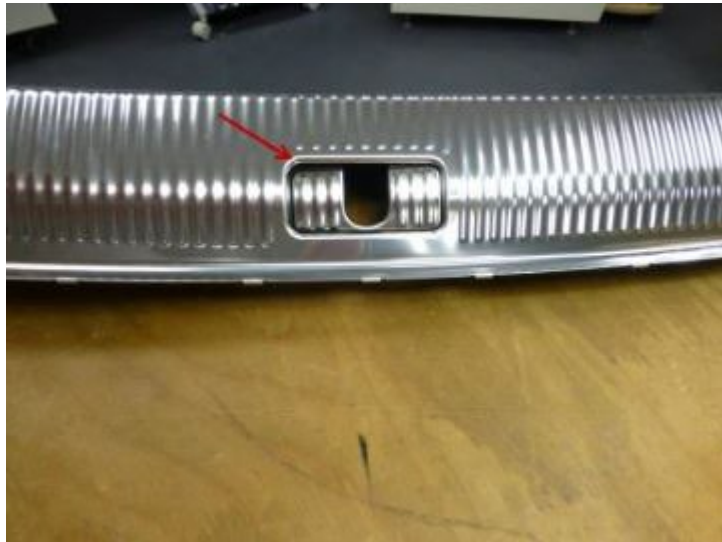
Figure 5. Damaged latch entry cover.
