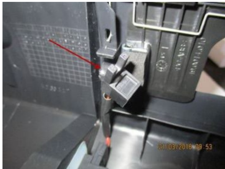
Figure 4. Loose G525 hall sensor.
