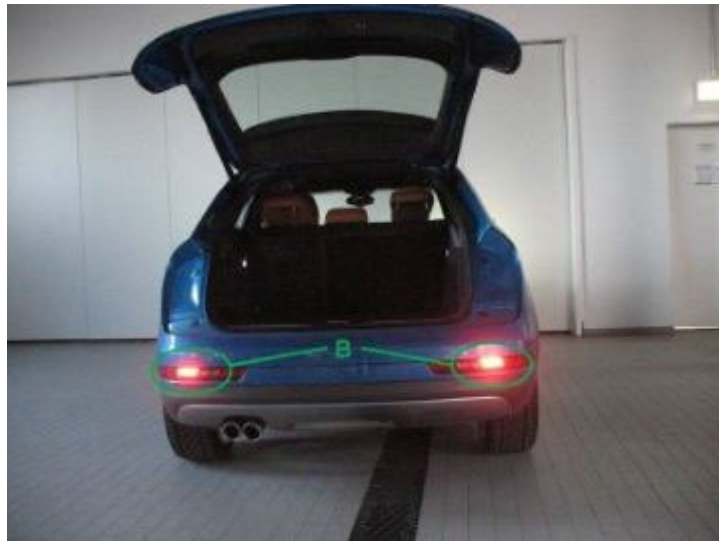
Figure 2. Rear lamp operation with rear lid open.
