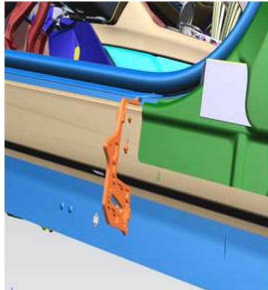
Figure 6. Side member cavity sound absorber.
