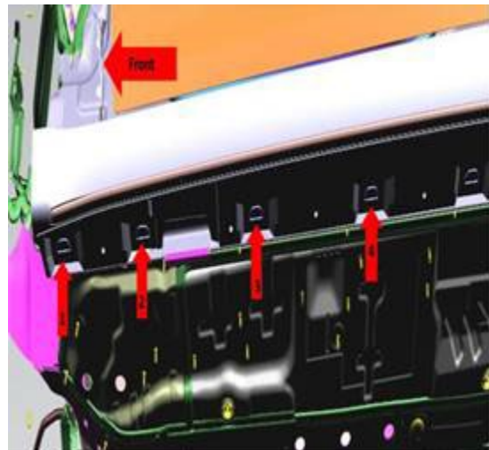
Figure 3. Sill trim fastener openings.
