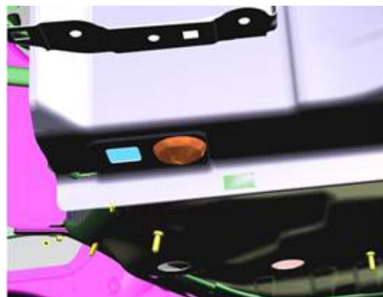
Figure 12. Drain plug on the front of the side member.
