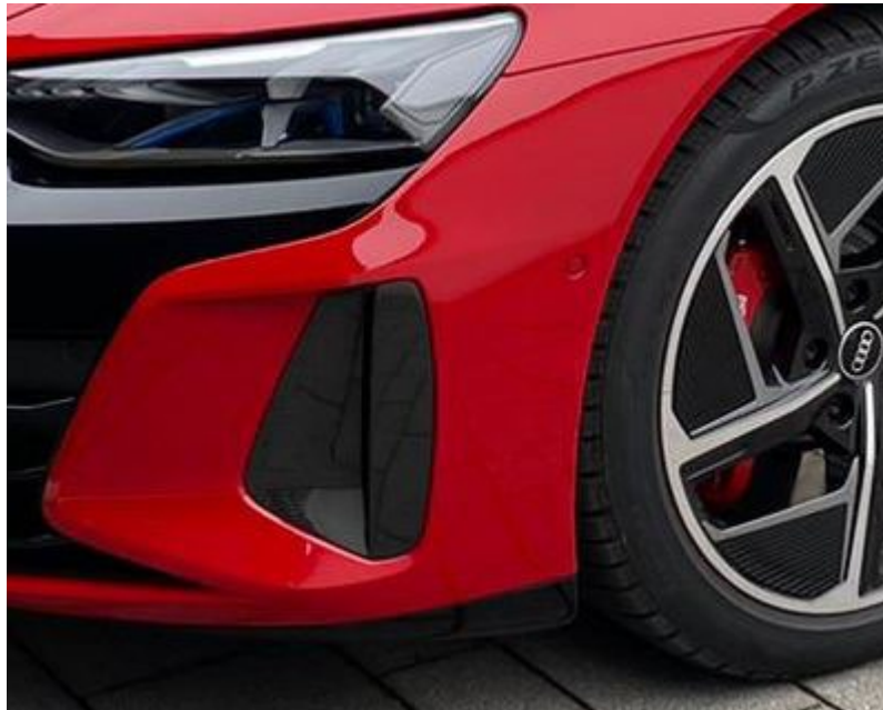
Figure 1. Side air duct.
