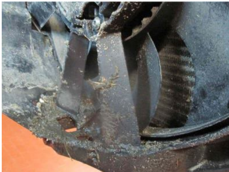
Figure 3. Radiator fan and fan shroud with debris accumulation.
