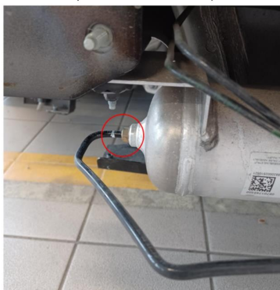
M189 – Compressed air tank – Pipe connections
