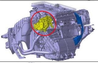
The heating and air-conditioning unit in the **G29**, left-hand drive (LHD) vehicles contain 2 servomotors total. **Driver Side** view
