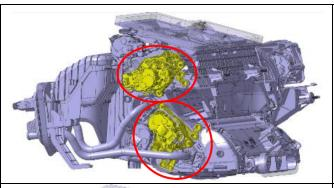
The heating and air-conditioning unit in F97 / F98 / G01 / G02 / G20 / G22 / G23 / G26 / G42 / G80 / G82 left-hand drive (LHD) vehicles contains 3 servomotors total. **Driver Side** view
