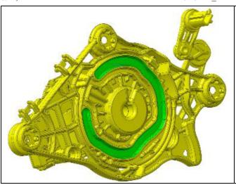
4. Remove the old grease on the gate disc of the kinematics (green area) with a clean cloth and use Unisilkon TK M1011 to regrease.
