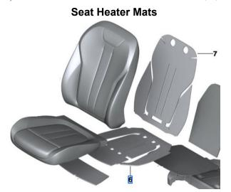
The seat heater mat (6) is controlled by the seat module.
