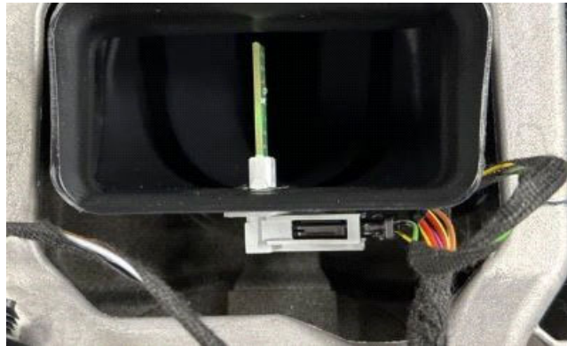
Figure 1. Harness routing prone to damage in assembly.
