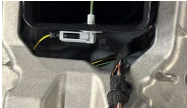
Figure 2. Corrected rear vent temperature sensor position and harness routing.
