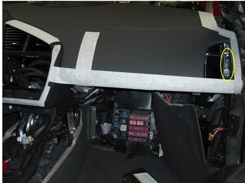
Figure 1. Right instrument panel vent removed.
