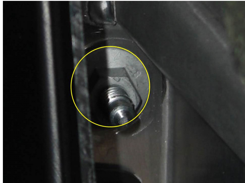
Figure 3. Instrument panel carrier nut to be marked.
