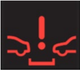
Figure 2. Distance warning light.
