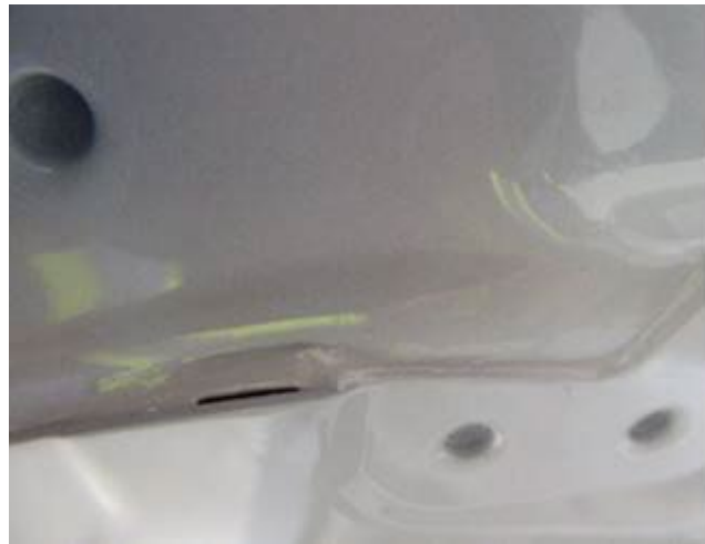
Figure 7. Close up view of the sealer flaw.
