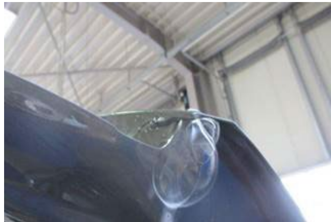
Figure 1. Bubble formation with compressed air applied internally.
