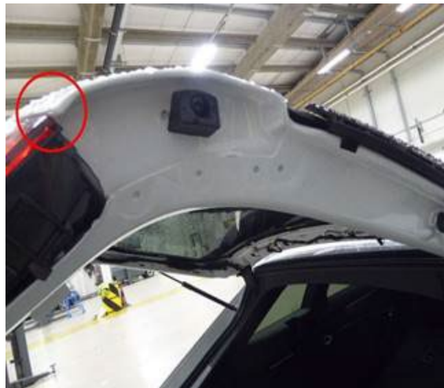
Figure 1. Bubble formation with compressed air applied internally.
