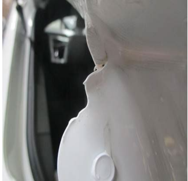
Figure 3. Possible sealer flaw area behind tail lamp.
