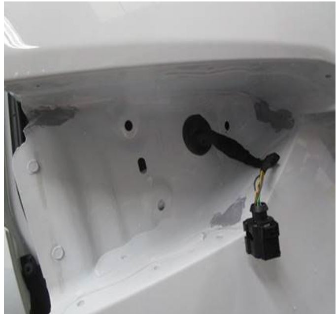
Figure 9. Concealed areas repaired with D 476KD1M2 or D 476KD1M3 sealant.
