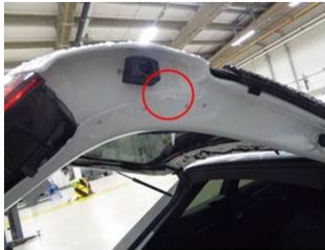
Figure 6. Sealer flaw on side of rear lid.
