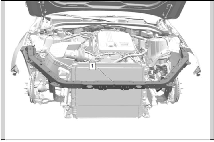
If a significant voltage drop is found, technician will need to remove and clean the Front Compartment Front Panel attaching points and fasteners(1), see below.
