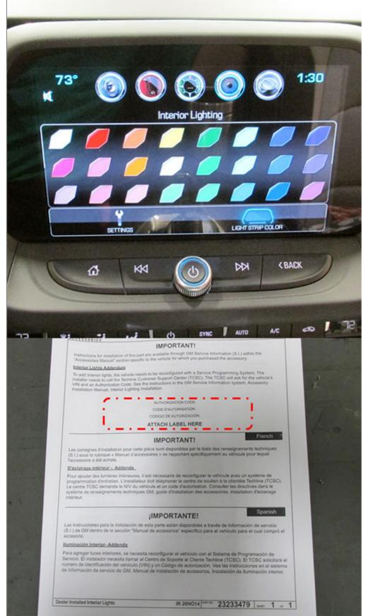
Vehicles equipped with the base radio (RPO IOB or IOR) do not require any programming. That is why the color selections are not available on the radio screen. This system uses a dashmounted switch to change the system's lighting colors. It is installed on the left hand side of the steering column. This switch can be seen in the photo below.
