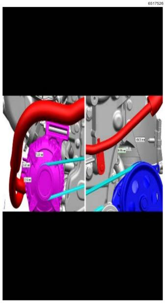
Verify the is proper clearance between the Batter positive cable and the alternator and water pump.
