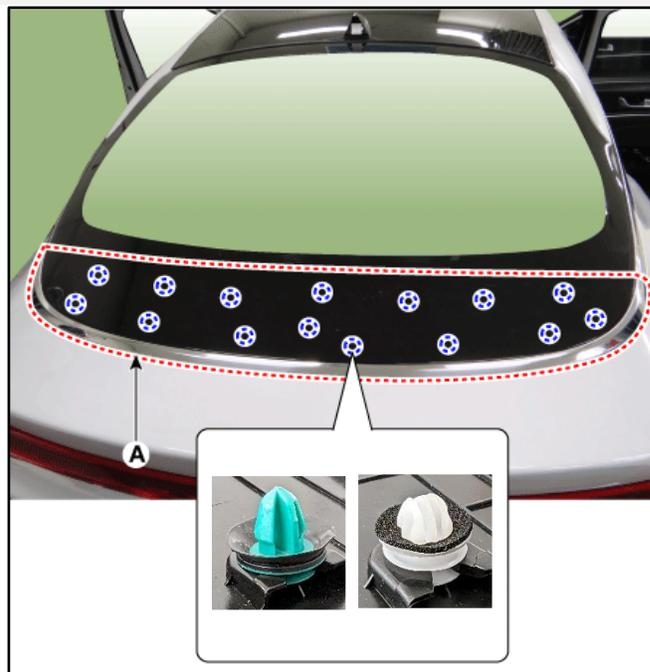
2. Carefully place the removed rear trunk lid garnish face down over a clean cloth to protect the gloss black painted surface.
