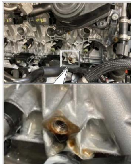
Example of an oil leakage
