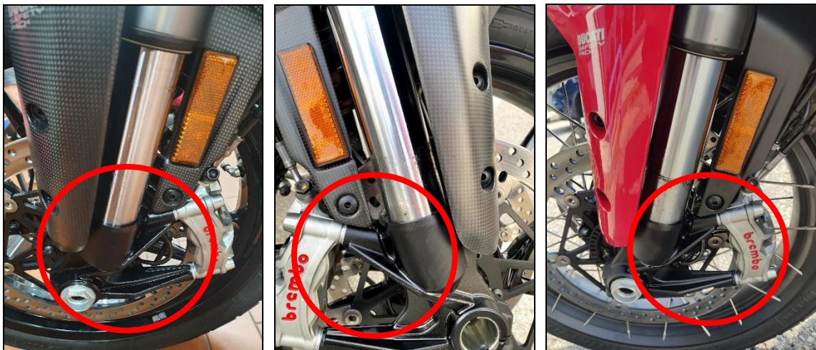
Example: Oil leak that has reached the fork axle lug
