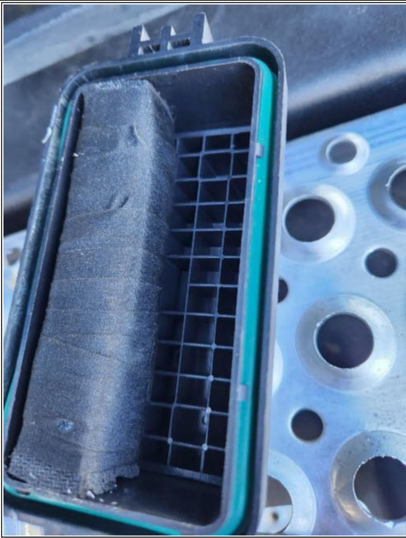
Figure 5: Foam Block Installed in PDM Cover
