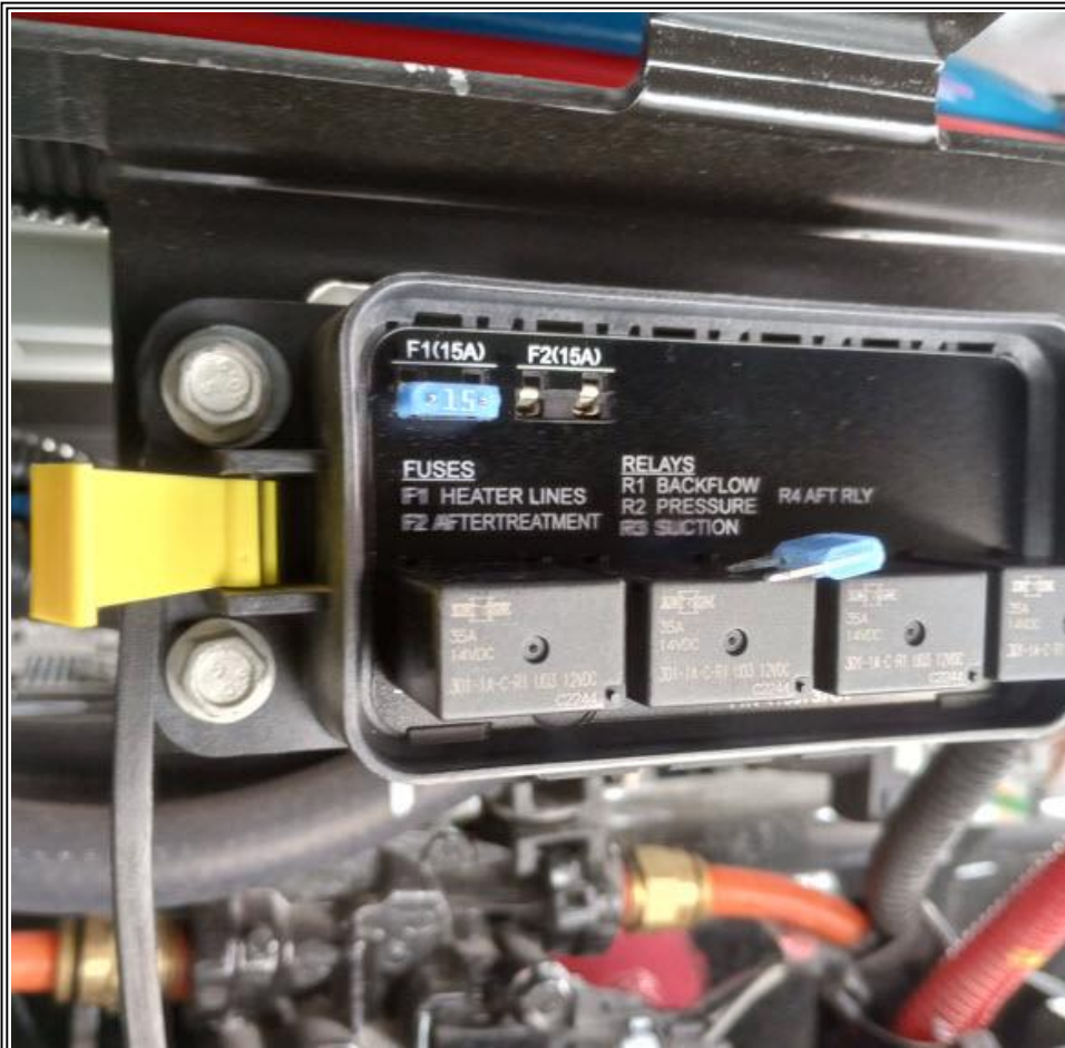
Figure 4: F2 Aftertreatment Fuse Loose in PDM Cover
