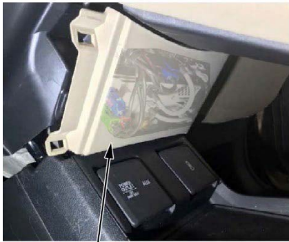
LOWER CENTER COVER (infotainment control unit located behind)
