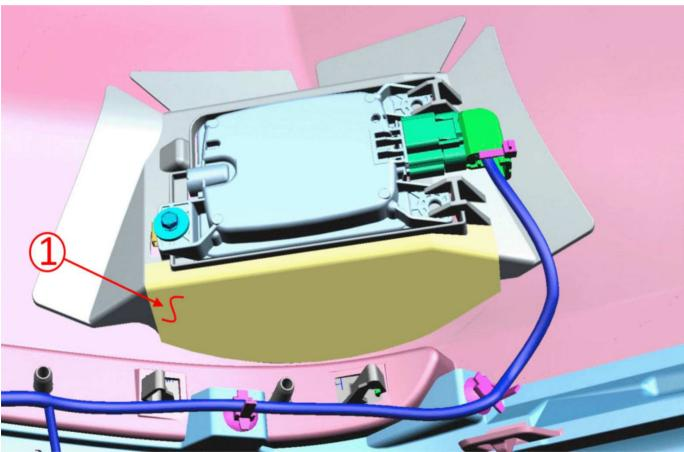
7. Peel the backing off the aluminum butyl tape (1) and apply to the bottom of the module making sure the area is completely covered as shown in the graphic above.
