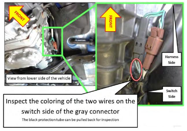
**STEP 5:** Apply the visual inspection results from **STEP 4** to the table below to verify the next course of action.
