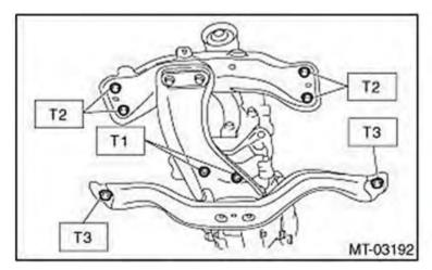
Torque Specification T1: 35Nm (25.8ft-lb) T2: 70Nm (51.6ft-lb) T3: 140Nm (103ft-lb)
