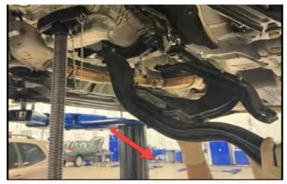
**STEP 14:** Loosen the mounting bolts securing the center heat shield and then CAREFULLY remove the heat shield toward the passenger side of the vehicle. Swing the rear portion of the heat shield out first and CAREFULLY thread the oxygen sensor wiring through the shield.
