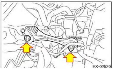
STEP 9: Set the transmission jack to support the transmission.
