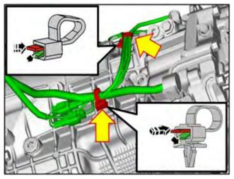
**STEP 19:** Disconnect the gray two-pin connector on the back-up switch harness.
