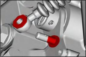
**STEP 31:** Install the cross member to the transmission with the two mounting nuts. Install the heat shield with the mounting bolts hand tight. Confirm the alignment is sufficient by adjusting the transmission jack if needed. Install the cross member to the vehicle body with the six mounting bolts. Torque the crossmember mounting bolts. Once the torque procedure is complete, the transmission jack can be removed.
