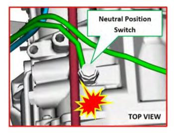
**STEP 22:** Loosen the back-up switch from the transmission case. Rotate the switch harness while turning the socket to prevent any excessive tension. The switch and the special tool cannot be removed together due to interference with the transmission case. Remove the tool before removing the switch.
