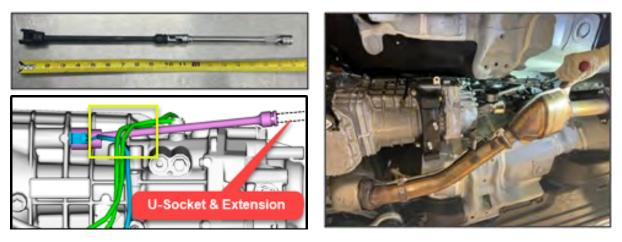
**CAUTION:** Confirm the socket is fully seated onto the back-up switch. Confirm the wires are not damaged by the socket.
