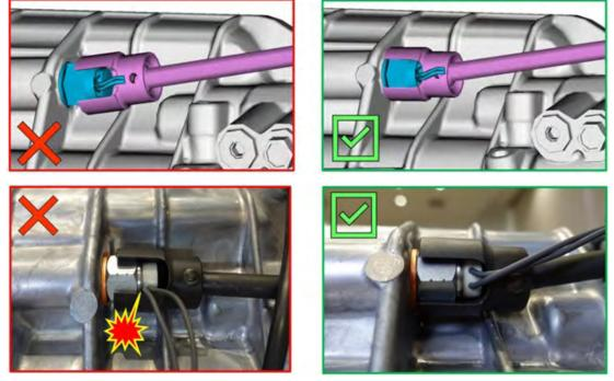
CAUTION: Take particular care not to damage the neutral position switch with the special tool.
