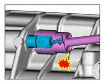
**STEP 23:** Install the new back-up switch with the new gasket. Rotate the switch by hand while turning its connector in order to avoid any twisting of the harness.
