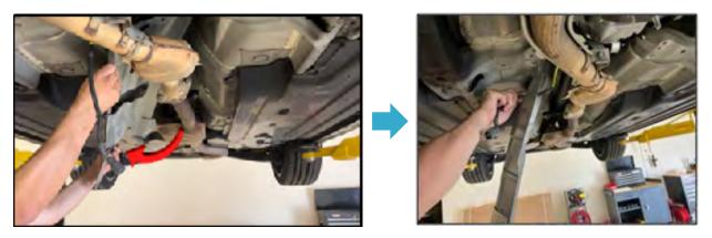
**STEP 15:** Remove the snap pin and washer from the reverse check cable. These parts will be reused and should be stored securely. Once removed, disconnect the cable from the reverse check lever.
