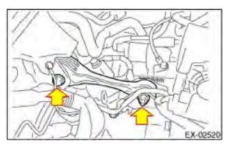
**STEP 35:** Reinstall the intercooler in accordance with the applicable Service Manual. Be mindful not to deform or damage the intercooler fins. For 2019MY S209 models, install the STI flexible Tower Bar. Refer to the <u>S209 Service Manual</u>.
