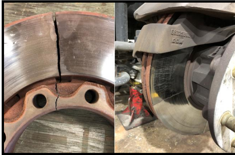
(Example of failed rotors)
