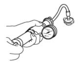
2.Apply pressure using the radiator cap tester.
