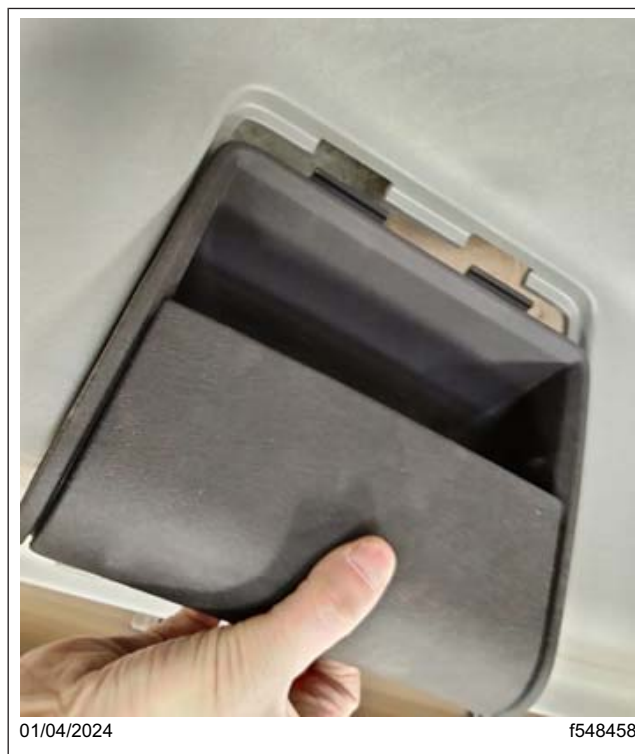
Fig. 13, Sunglasses Pocket Removal from the Overhead Console
