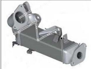
For the eligible vehicles, BMW of North America, LLC (BMW NA) is extending the limited warranty for the vehicle's **Exhaust Gas Recirculation (EGR) Cooler** (shown) to:
