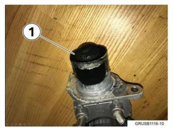
Remove the EGR valve and check for jamming (valve is normally sprung closed).
