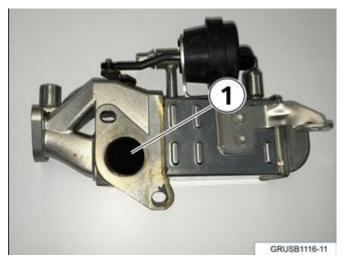
12. Inspect the cooler by-pass flap (1).
