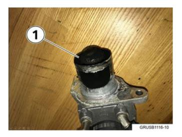
8. Remove the EGR valve and check for jamming (1) (valve is normally sprung closed).
