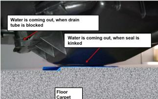
If an outflow of condensation is visible, the condensation drain must be replaced.
