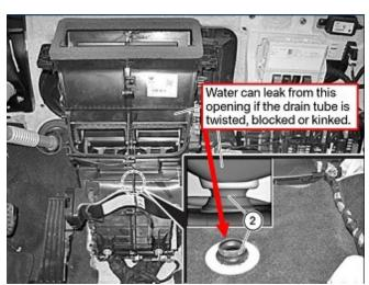
Then perform a visual check, with an endoscope, if possible, to check whether the sealing crown has been folded down / kinked / deformed.
