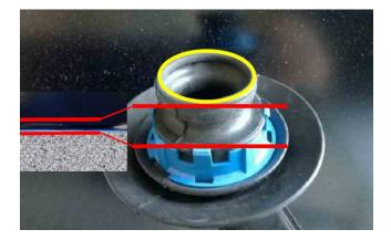
When replacing the drain, treat the sealing crown in the upper area with a lubricant (for example: silicone lubricant: Part number 83 19 2 240 251). Make sure the drain is not deformed and install parallel to the floor and carpet.
