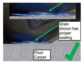
After installation, check for the correct application of the sealing surface / contact surface.
