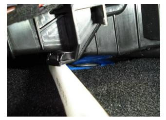
Using a lever, press the carpet down to obtain a clear view of the condensation drain sealing crown to the heating and air conditioning unit.
