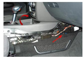
Disassemble the footwell trim on the driver's / passenger's side; remove the center bottom left / right instrument panel trim (driver's and passenger's side).
