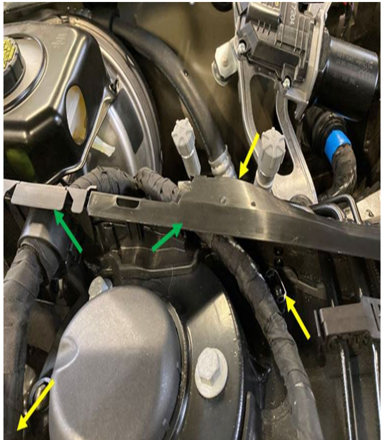
Figure 1: Plenum chamber covers (green arrows).
