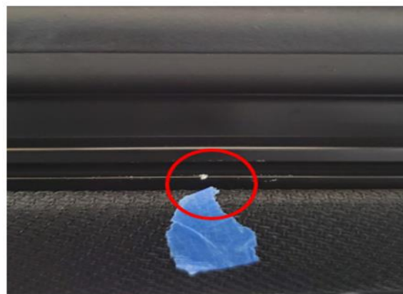
Knock off any vertical burr on horizontal surface and touch up with a black paint pen or permanent marker.
