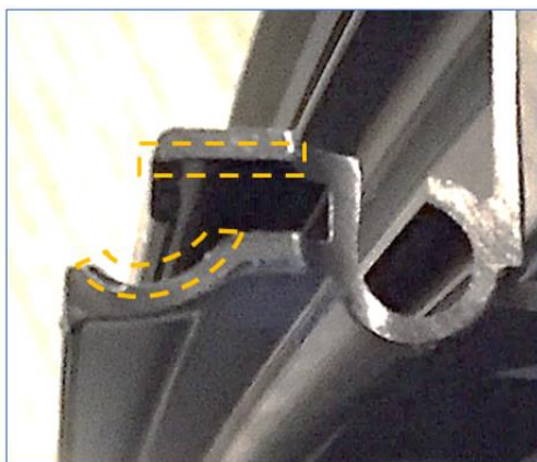
Run a round pick across these two edges to break the edge.
