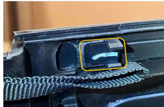
Clip attached to panel with a press fit rib on the back into a slot on the panel. Glass supplier glues the rib with cyanoacrylate glue.
