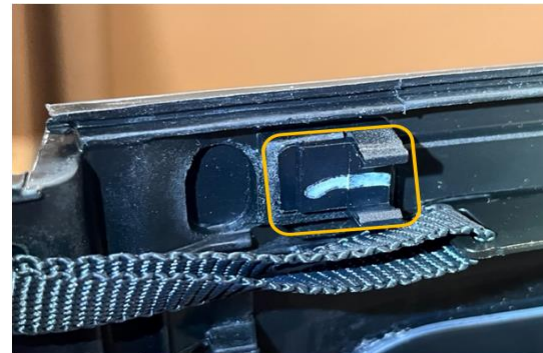
Clip attached to panel with a press fit rib on the back into a slot on the panel. Glass supplier glues the rib with cyanoacrylate glue.
