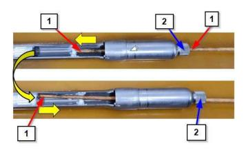
3. Through the opening of the steering wheel shaft (2), ensure the even distribution of grease in the internal gearing of the steering wheel shaft.
