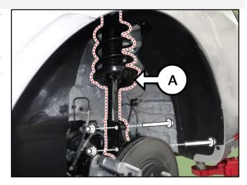
Disassemble one of the front strut assemblies
