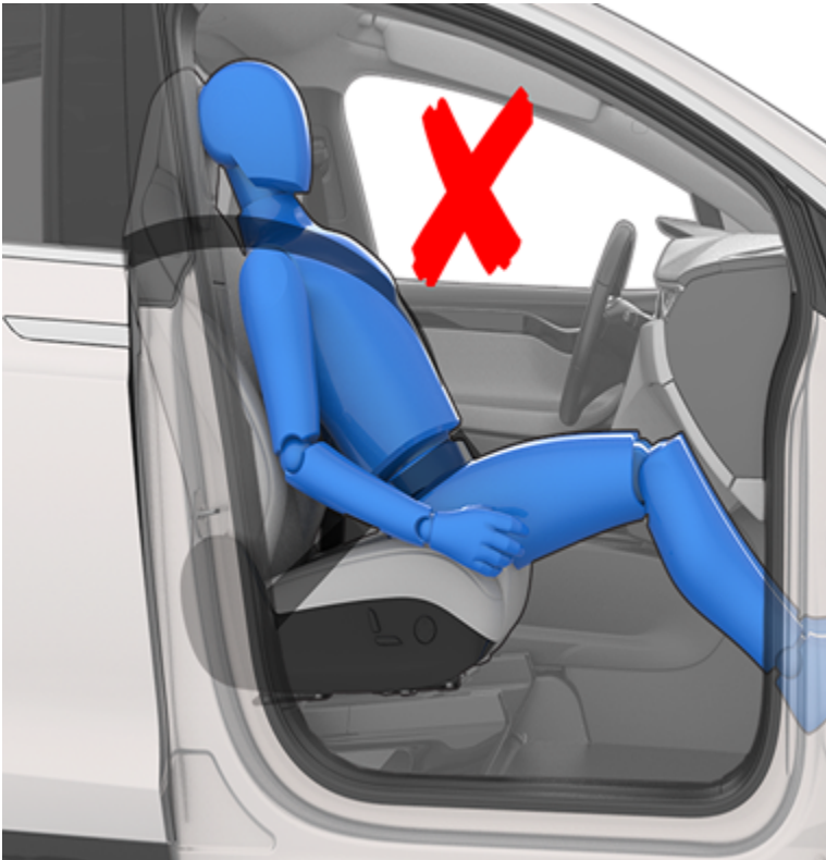
Incorrect seating position - the passenger must not recline the backrest to a laying down position when the vehicle is moving:
