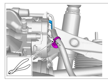
Cut following the dotted lines. Loosen the wiring harness or move it to the side.
