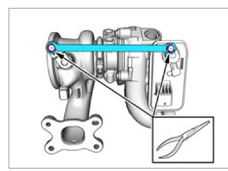
Install the marked component. Install the clip(s).
