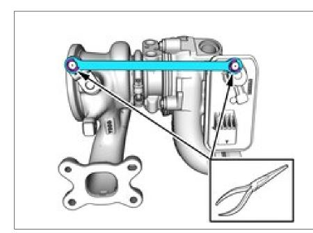
Install the marked component. Install the clip(s).
