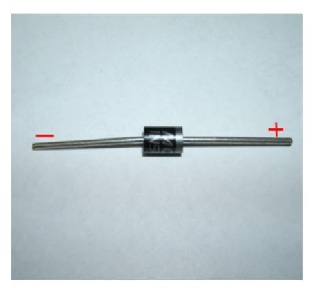
Install a diode, P/N 12112422, across the coil of the solenoid. It is important that the striped end of the diode be connected to the positive terminal of the coil and the other end of the diode be connected to ground.
