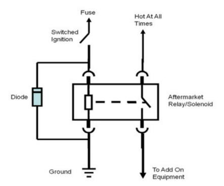
Install a diode, P/N 12112422, across the coil of the relay. It is important that the striped end of the diode be connected to the positive terminal of the coil and the other end of the diode be connected to ground. Be sure to insulate the diode with heat shrink tubing before installing.
