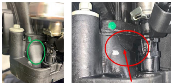
Fig. 2 Crack Shown Up Close
