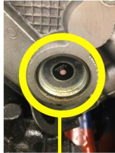
Overheated Pink Sensor 255°F Coolant Temp
