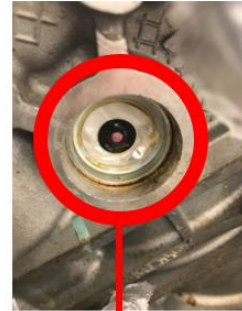
Overheated Red Sensor +255°F Coolant Temp
